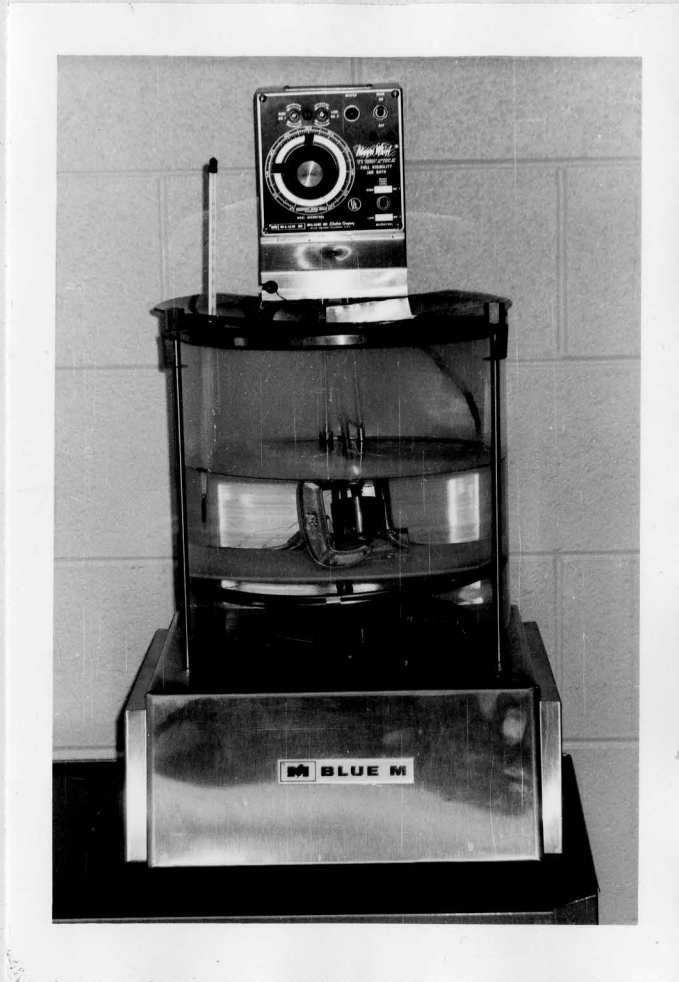
Fig. 6 Constant temperature water bath with die in place
